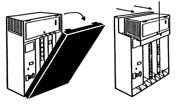
Figure 2 Removing the Front and Top Covers From the control Unit
